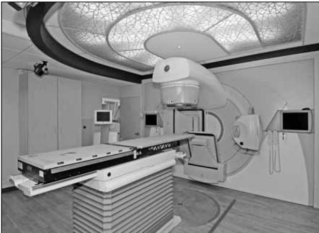
Figure 1: Linear Accelerator
